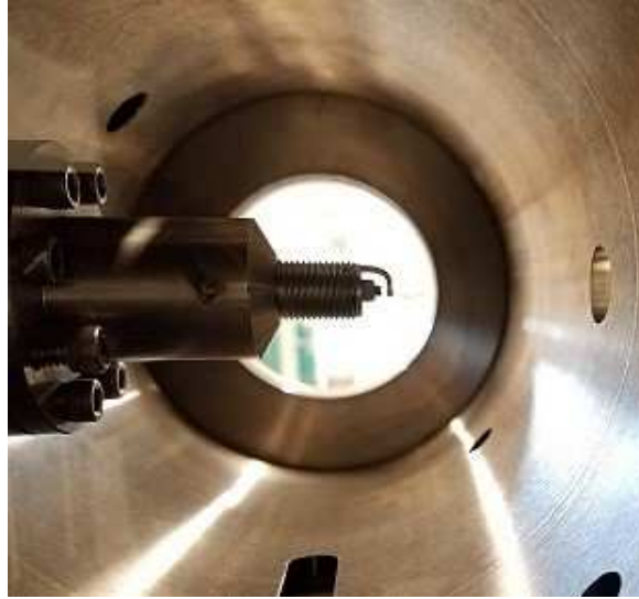
Figure 2.5: Spark plug mounted in combustion chamber for spark ignition experiments.
